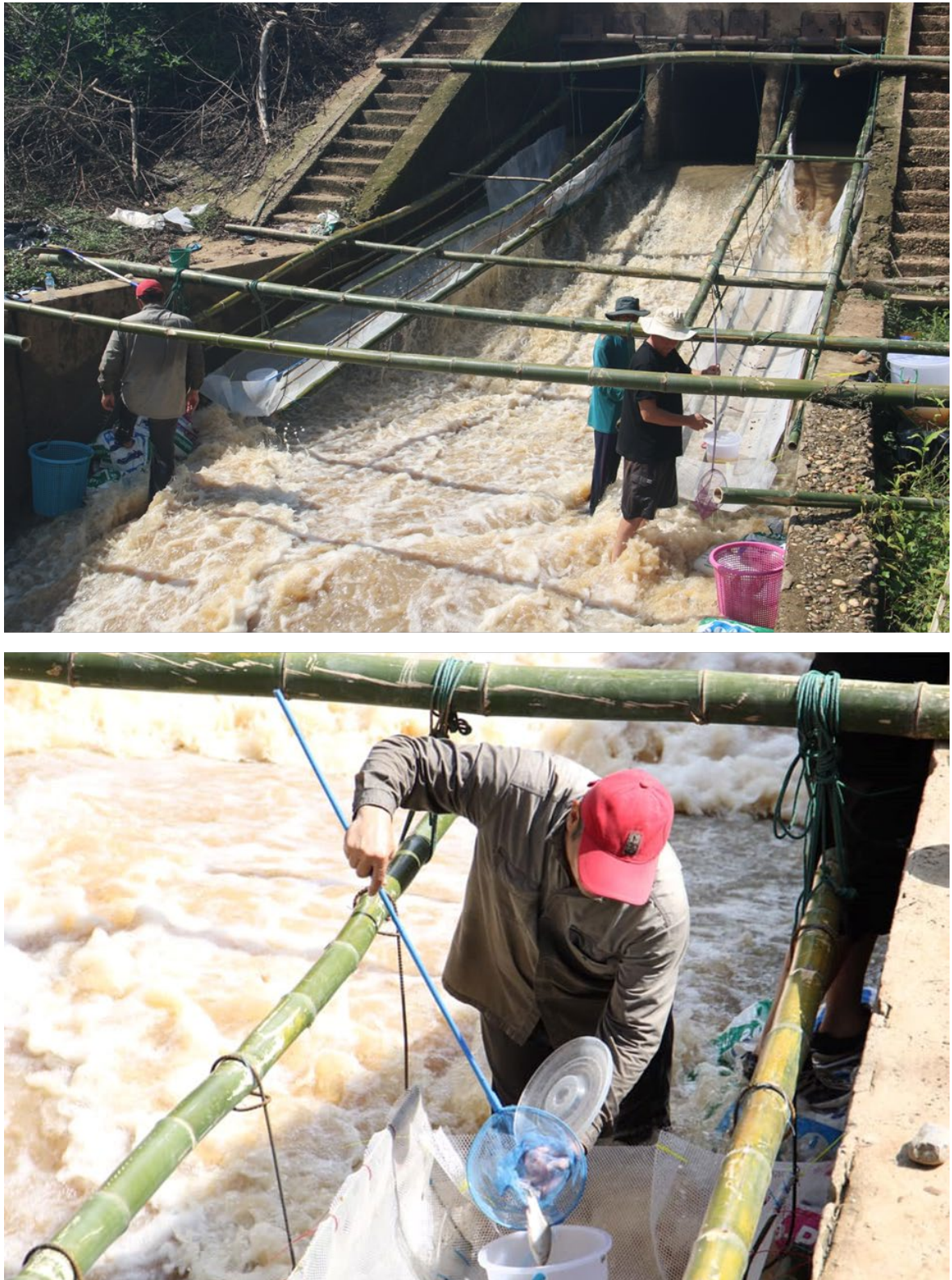
Figure 22. Lee traps were constructed in the Pak Peung spillway to capture fish that had passed the undershot or overshot gates. The Lee traps resulted in considerably less damage to fish than the original approach of using fyke nets. As water flows along the Lee trap it falls through the mesh, reducing the energy of flow and allowing every single fish to be captured. To further reduce the chances of net damage, the traps were constantly manned and fish removed and put in a bucket of water as soon as they were captured.
