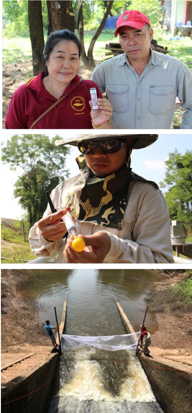
Figure 17. Sensor Fish (top) were used to evaluate the hydraulics of the Pak Peung gates. They were deployed upstream of the structure by trained staff (middle) and recaptured after passing the gates using a net (bottom).
