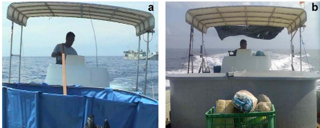
Fig. 6. a. Vinyl on-board holding tank (2 m 3 ) used until 2010. b. Covered fibreglass holding tank (2 m 3 ) used with oxygen in 2010.
