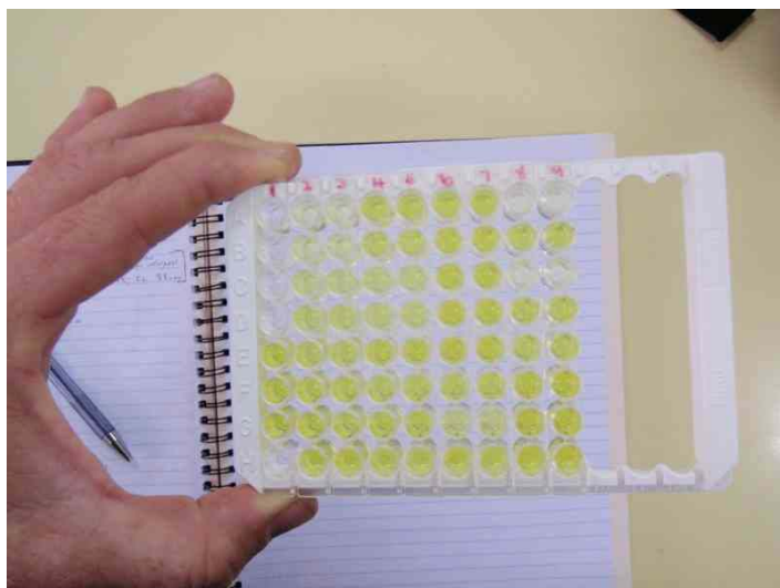
Fig. 9. 96 well 11-Ketotestosterone EIA plate used to determine sex of yellowfin tuna broodstock at RIM Gondol.
