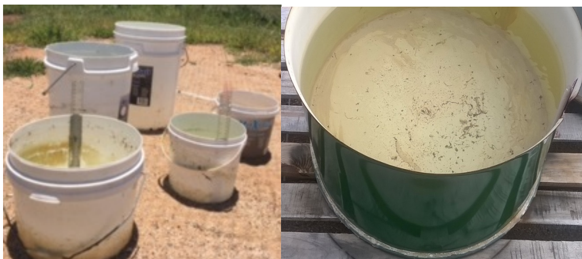
Figure 29. Different containers used as evaporation pans showing various sized plastic buckets (left) and a part 200 l drum (right).
