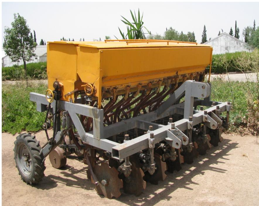
**Plate 2** INRA designed (CRRRA Settat) ZT drill unit manufactured in collaboration with Atmar. 32 units have been made to date (An equivalent unit was separately developed by the Agro-equipment and Energy Department at IAV II)
