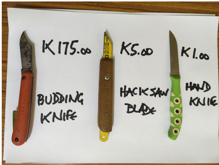
Plate 7.10. Steps towards appropriate low-cost technology in budding knives, with expensive imported budding knife on the left.
