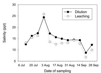
Figure 13. The soil solution salinity (ppt) at Cai Nuoc where conventional farmer practice of salinity management (dilution) was compared with enhanced leaching using platform bunds (leaching).
