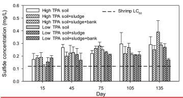
Figure 18. Sulfide concentration (mg/L) in water columns over soil, sludge, and sludge with eroded bank soil for two farms (high TPA and low TPA). Error bars represent standard deviation. The  $LC_{50}$  sulfide concentrations for shrimp are indicated by a horizontal line (Goppakumar and Kuttyamma 1996).
