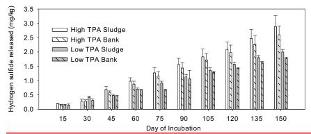
Figure 17 Release of hydrogen sulfide ( $H_2S$ ) (mg/kg) from incubated soil of earthen banks or ditch sludge taken from high or low total potential acidity (high TPA and low TPA, respectively) farms. Error bars represent standard deviation.
