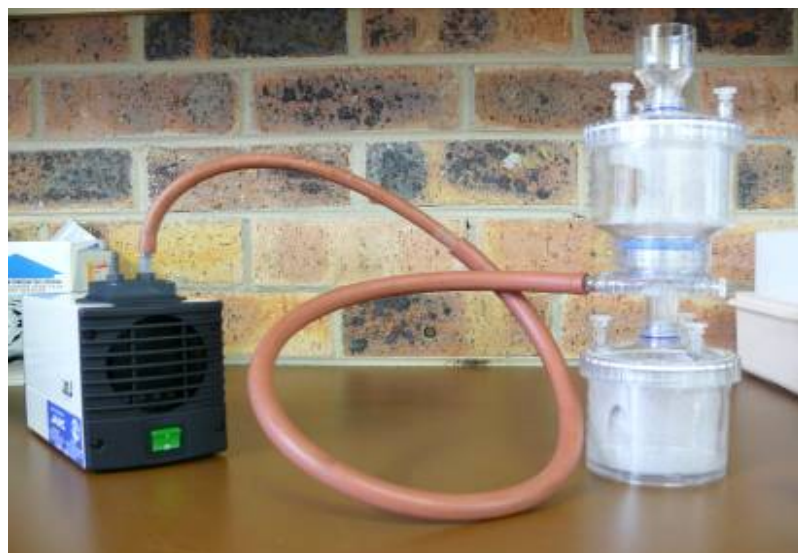
Figure 4. Filtration system and vacuum pump
