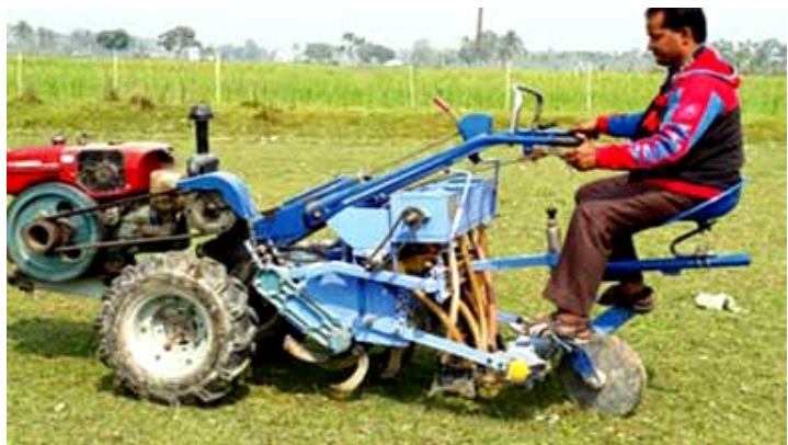
Fig. 4: The VMP attached with 2-wheel tractor in operation
