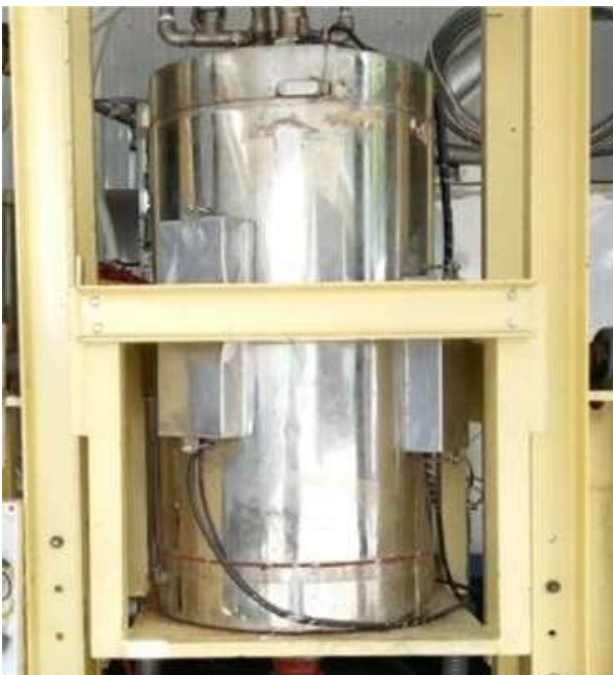
Figure 11. Hydrothermal carbonisation (HTC) of wet organic wastes in a low-temperature pressure reaction vessel.
