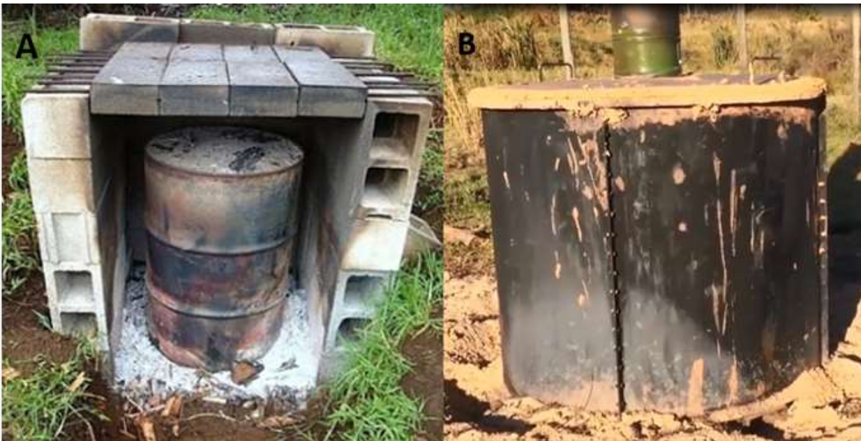
Figure 10. Typical kilns used to produce biochar.
