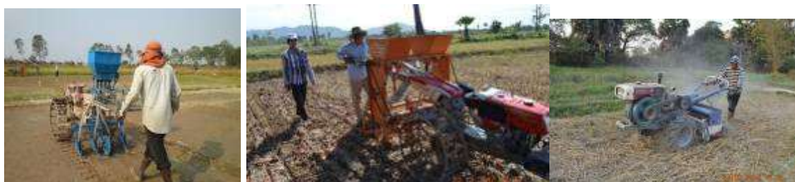
Figure 6.4. Seed drills selected and evaluated in the project (from left to right: Thai disc drill, Cambodia-made Rogro tine/press-wheel drill, Chinese rotary till drill 2BFG-100).
