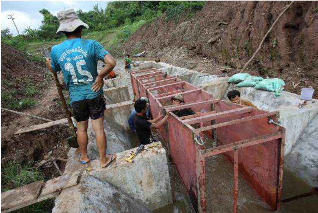
Figure 5. During high Mekong levels the experimental unit was set up within the permanent fishway channel which provided more control over discharge and depth (Photo Jim Holmes).
