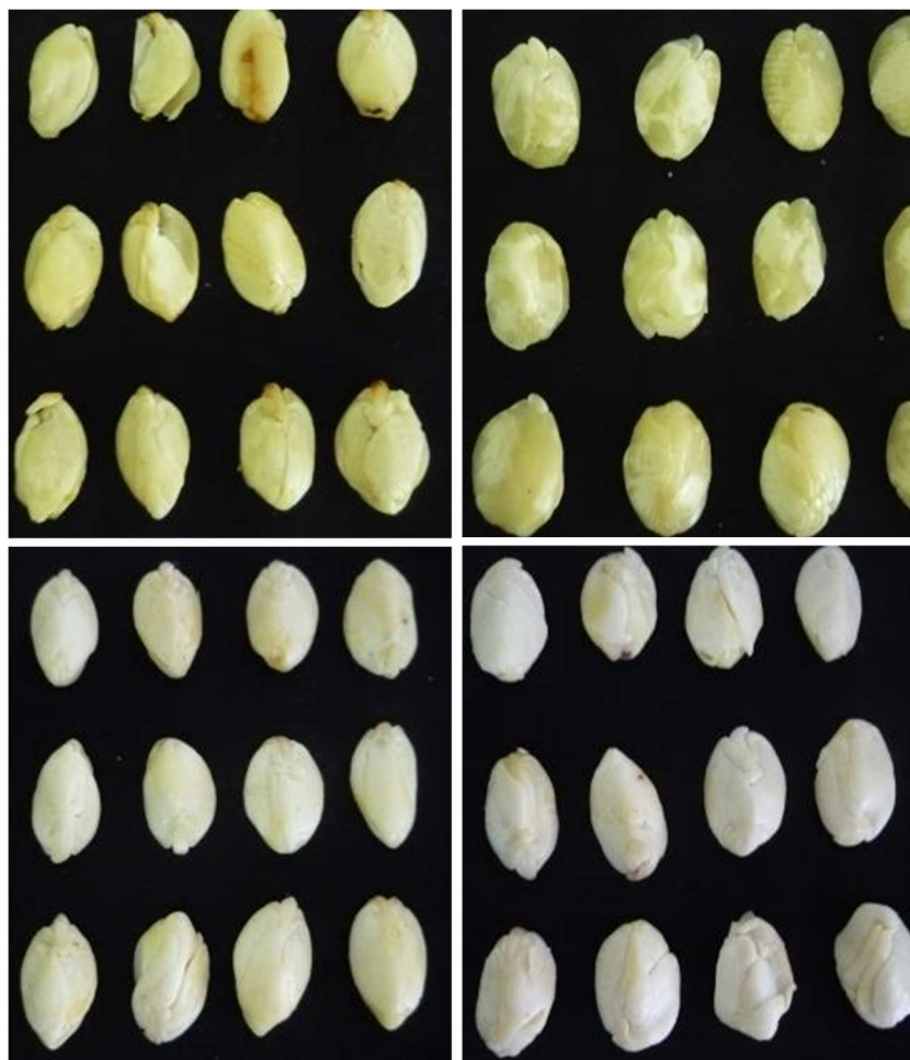
Figure 7. Colour of Canarium kernel dried for 6 hours at 80°C (top left), 60°C, 50°C and 40°C (bottom right).
