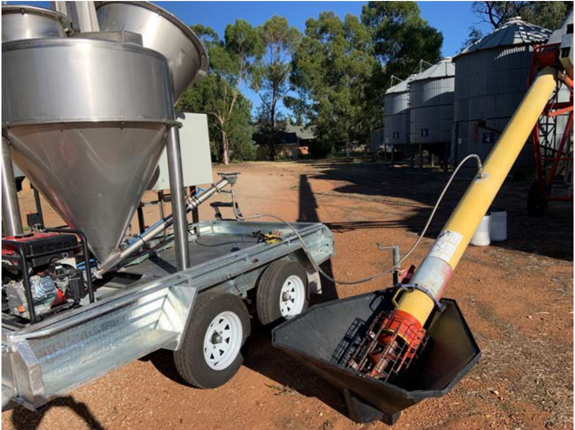
Image 1: SAS field application device that feeds an aerosolised stream of SAS into a moving grain flow being fed by a hopper fitted with an auger
