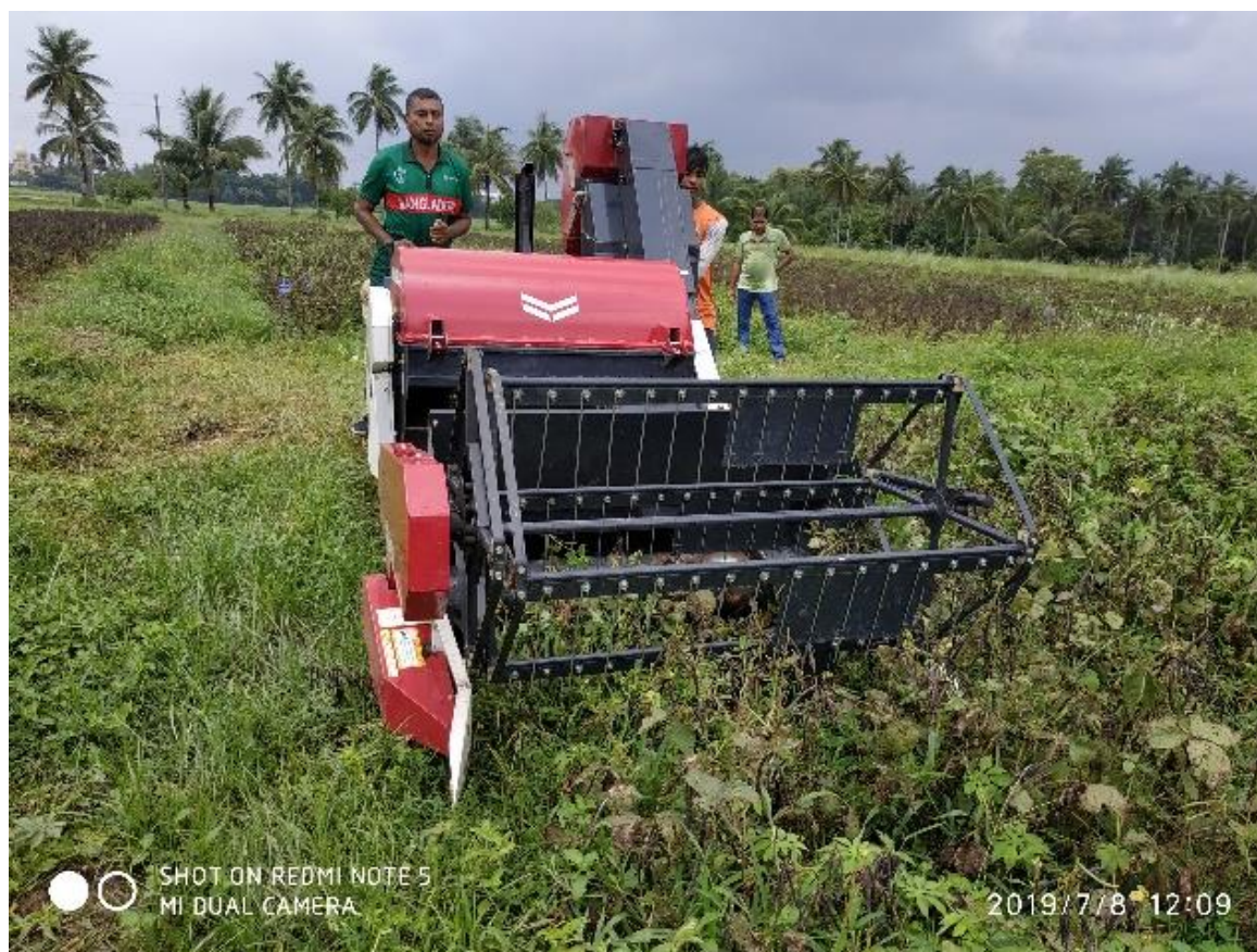
Figure 19. Machine harvesting field of mungbean at BARI Ishwardi, Bangladesh
