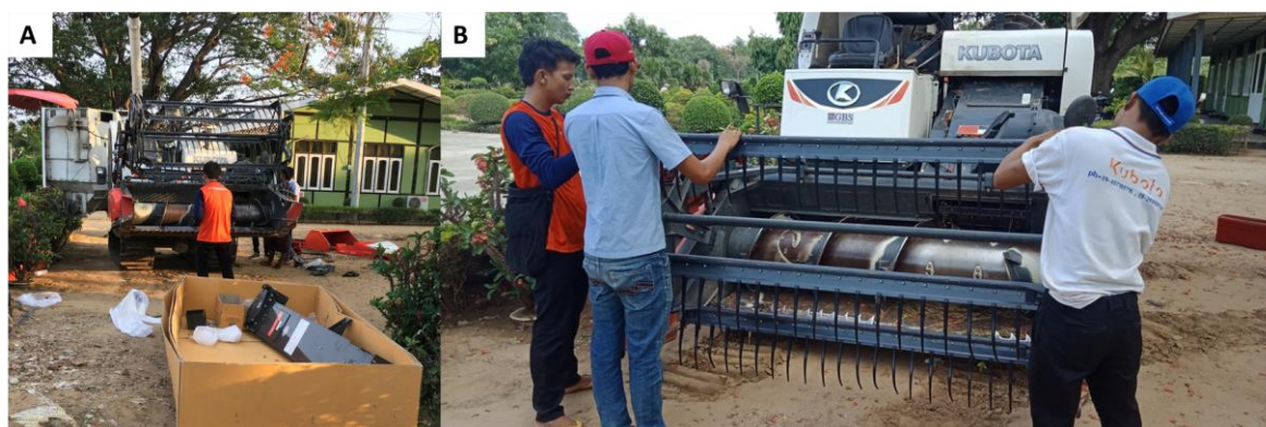
Figure 17. Installing bean kit on Kubota DC 70G combined harvester in Myanmar.
