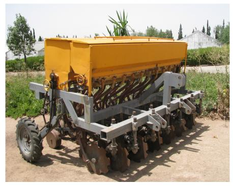
**Plate 2** INRA designed (CRRA Settat) ZT drill unit manufactured in collaboration with Atmar. 32 units have been made to date (An equivalent unit was separately developed by the Agro-equipment and Energy Department at IAV II)
