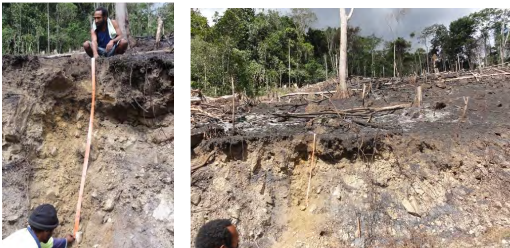
Plate 19 Soil Profile ACIAR SP10 and surrounds indicate moderately deep boulder rich colluvial soil profile exposed in road cutting. Soil is derived from sandy facies of the Owen Stanley Complex. Note new garden being prepared at the site via slash and burn methods.
