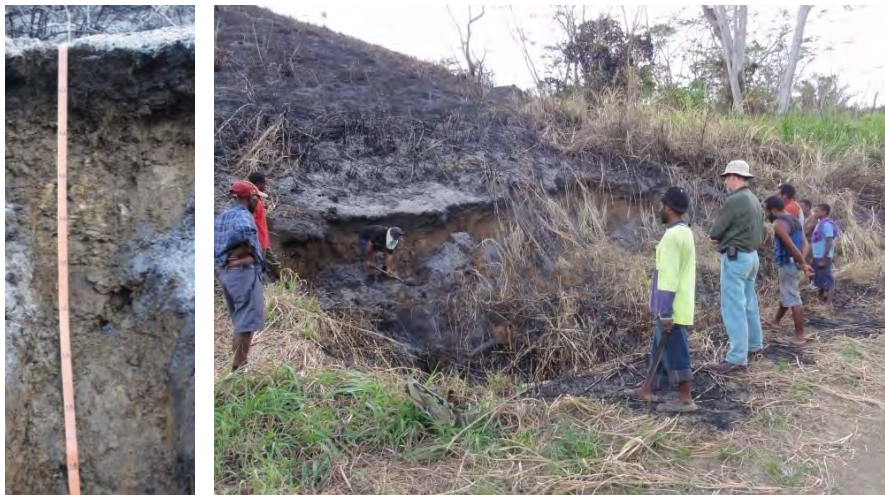
Plate 20 Soil profile (ACIAR SP11) - Deep fine textured colluvial soil (Vertosol) exposed in road cutting. Soil probable forms from debris from the pelitic phyllites (clayey sediments) of the Owen Stanley Complex.
