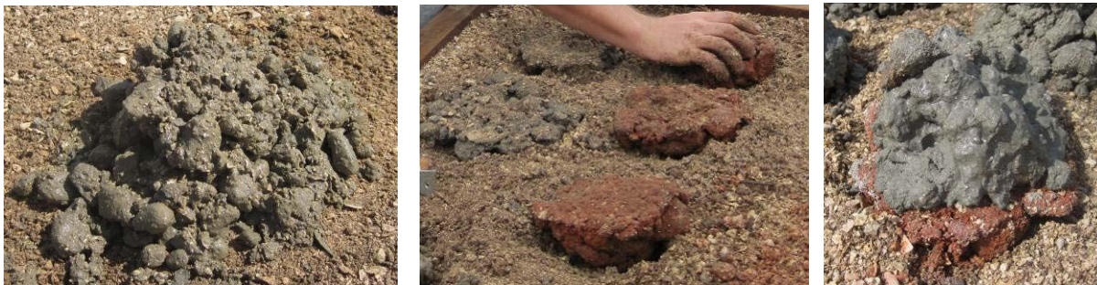
Figure 6. Tongan round-rock method of making an artificial rock composed of two semi-spherical halves concreted together. (a) First half rock, (b) hardened half-rock turned upside down in sand depression, (c) Second half-rock cemented on top. Note, one half-rock was made without red oxide.
