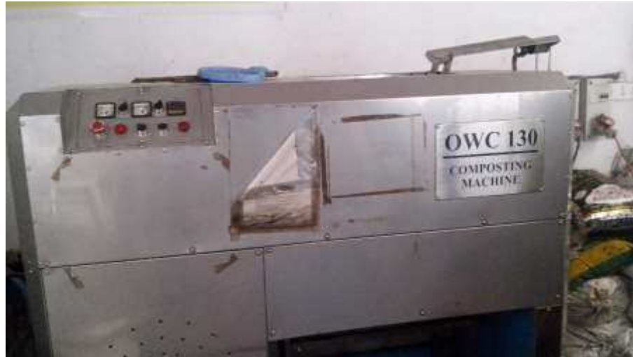
Pic. 4: Like with the 'Berkley Rapid Composting' the waste is scrapped to smaller bits using this shredder, at "Kasa to Rasa" unit – Saahas, urban Bangalore
