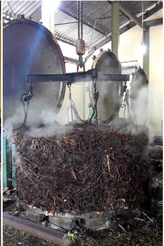
IMAGE 37 Three 2-tonne-capacity pots and the gantry crane for loading and unloading at the cajuput distillery at Sendangmole, Gunungkidul Credit: Prastyono
