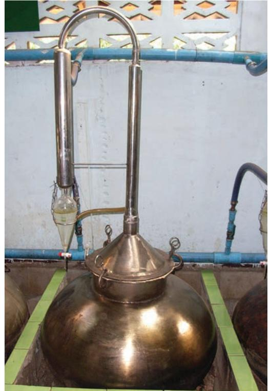
Figure 12.5 Sandalwood oil distillation units where chipped wood is treated with steam under pressure to release the oil from within
