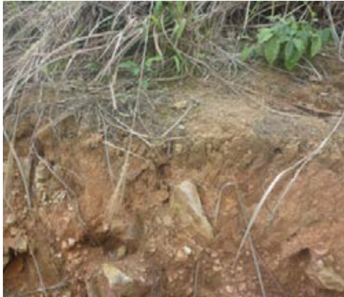
Photo 26. Shallow soil profile on sloping site with high proportion of large and small stones close to the soil surface, Guangxi province
