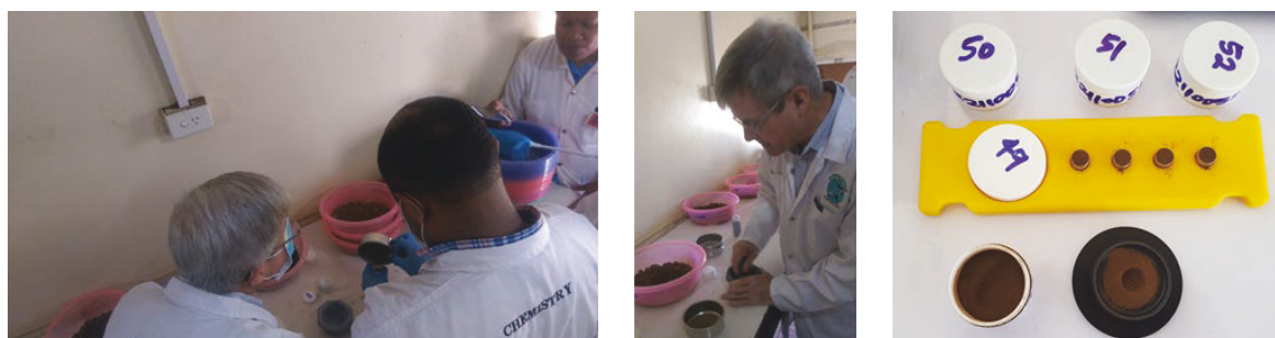
Figure 5 MIR soil specimen preparation in quadruplicates.
