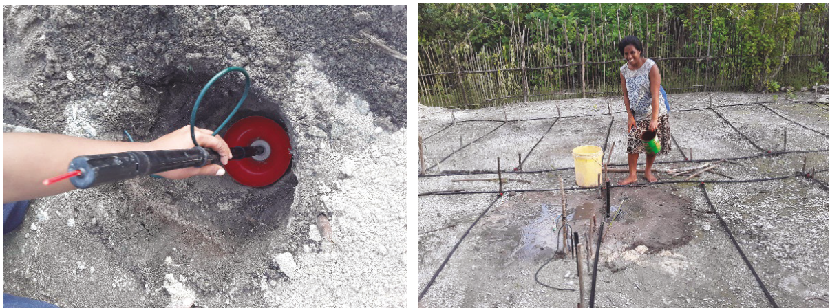
Figure 17. ALD staff installing Fullstops at the field trial and checking the Fullstop Installation
