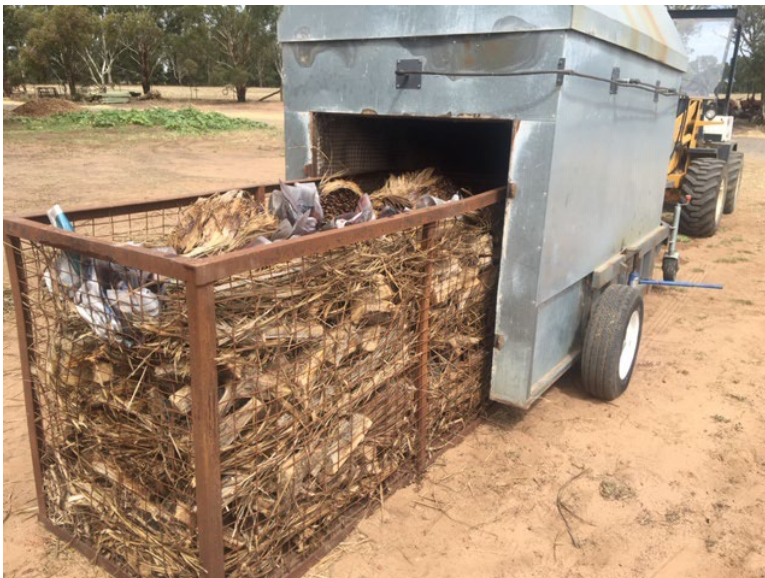
Figure 1.3.2. The Big-Roo unit being lowered onto the feedstock crate containing the oil palm trunk and fronds, ready for pyrolysis. The rear door is attached to seal the unit prior to ignition.
