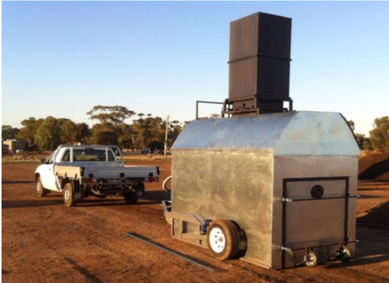
Figure 1.3.1. The 'Big-Roo' batch pyrolyser mobile unit used in this study.
