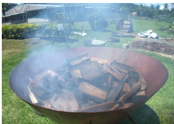
Figure 1.3.3. The Kon-Tiki kiln manufactured in PNG for this project by NBPOL personnel with an oil palm trunk feedstock undergoing pyrolysis.
