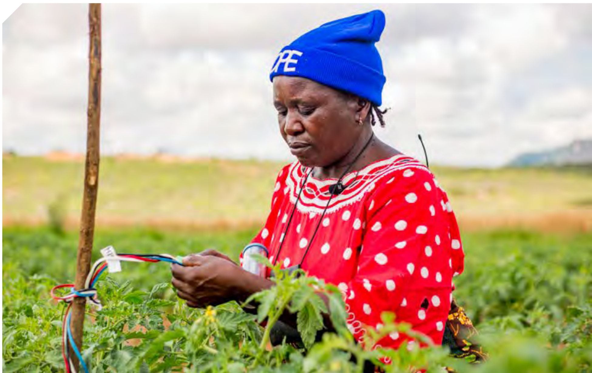
Ms Anatalia Kilienyi, a farmer from Kiwere Irrigation Scheme in Tanzania, sets up the Chameleon soil moisture monitoring device in her tomato crop. In pilot schemes in Malawi and Tanzania, irrigators using the device to manage irrigation timing reduced water use by 50% by extending the intervals between irrigation. Photo: ACIAR | 2021
