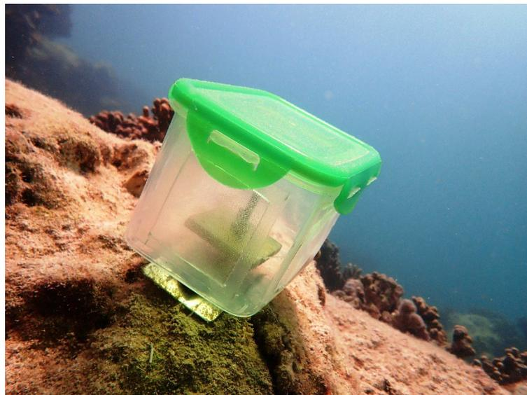
Figure 7.35. Settlement tile inside the settlement chamber attached to the reef substrata.
