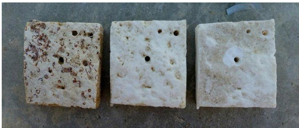
Figure 7.45. Examples of a settlement tile cut from dead plate *Acropora* spp. (left) and 3D printed replicas from PLA (middle) and ABS (right). (Image: Katy Horan).
