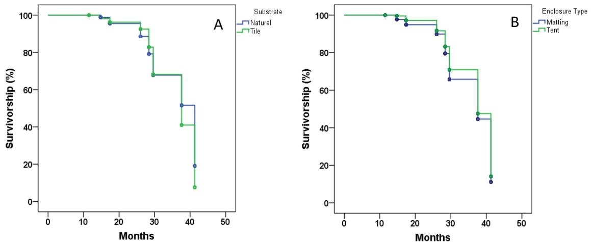
Figure 7.24. Kaplan-Meier survival curve of *A. millepora* corals that were settled onto degraded reef plots at Magsaysay reef (A) natural substrata and tiles, and (B) on the matting and tent treatment.
