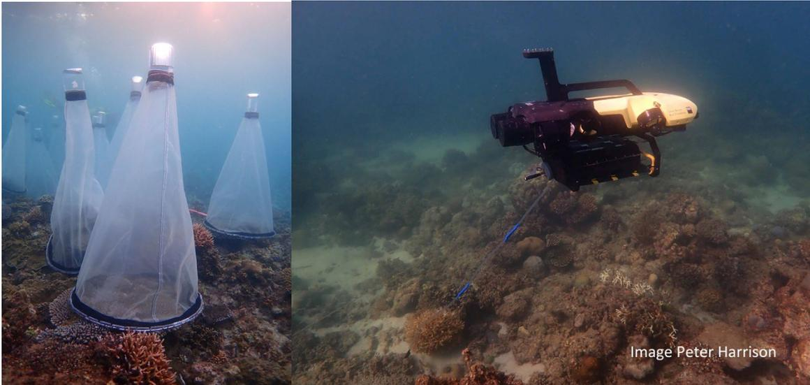
Figure 7.29: Coral spawn collection cones placed over 2013 *A. tenuis* restoration colonies just prior to spawning (left image), and LarvalBot dispersing larvae onto degraded reef sites along GPS controlled pathways in April 2019 (right image) (Images: Peter Harrison).
