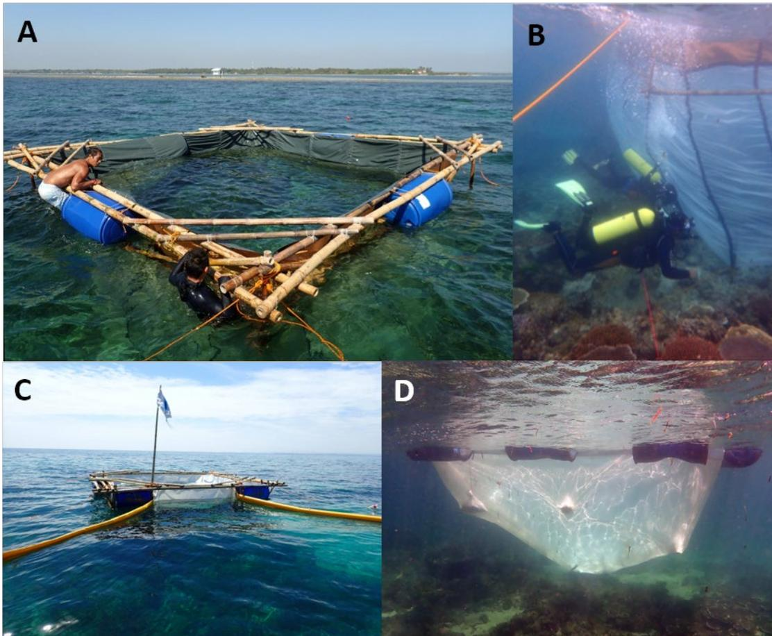
Figure 7.4: A prototype 5 × 5 m floating bamboo frame larval rearing pool deployed on Magsaysay reef in 2016 (A), and the submerged mesh curtain attached to the bamboo frame on reef site (B). Spawn catcher with booms attached to bamboo frame in 2017 on Magsaysay reef (C), and 2018 larval rearing net deployed under a floating steel frame (D) (Source: Harrison et al. 2021).
