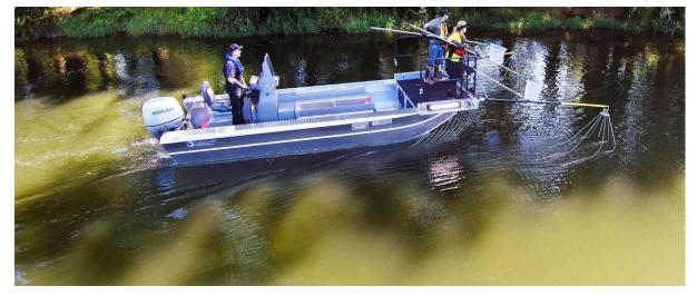
Figure 4. A large water electrofishing vessel in action. Electrofishing vessels work best when water has conductivity levels within an optimal range (usually 50–1000 micro siemens).
