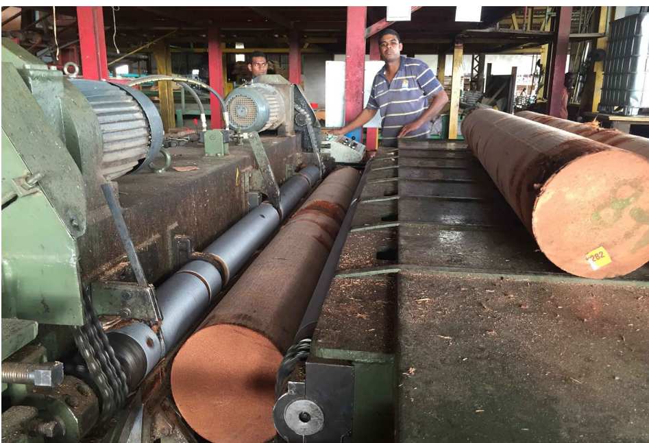
LEFT ACIAR-supported research has developed new ways to process coconut logs that allow them to be milled for veneers and other engineered wood products. Photo: QDPI
