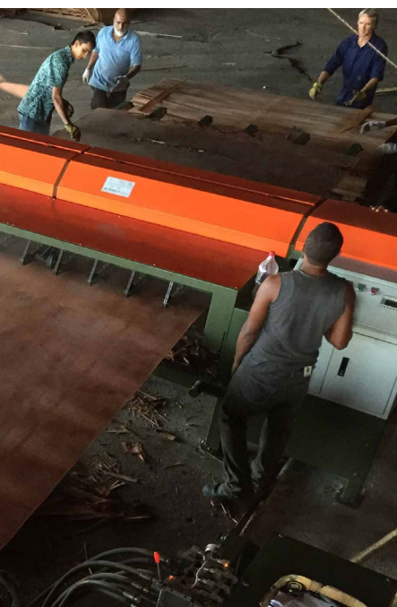
LEFT A coconut log being peeled in a spindleless lathe. Photo: QDPI
