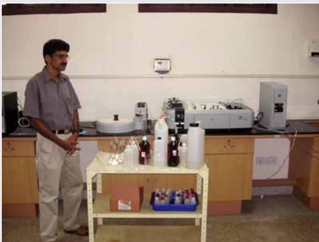
Dr Muralidharan with a newly commissioned segmented flow analyser in the central analytical facility of the Kerala Forest Research Institute
