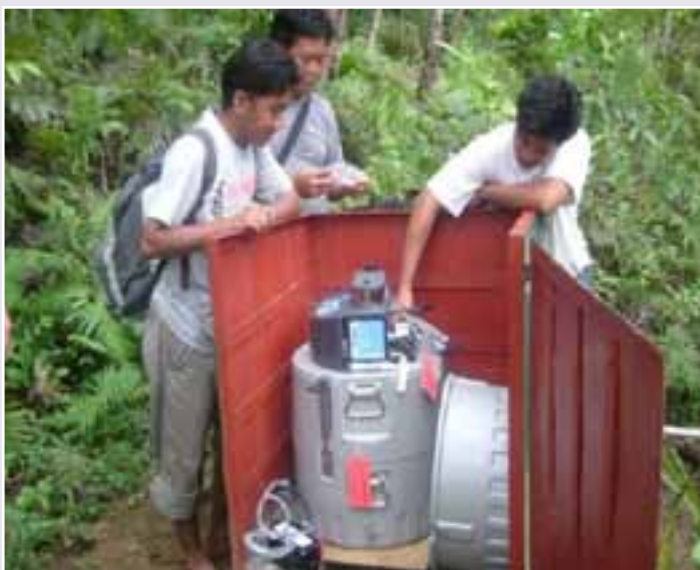
Staff from the Philippine Bureau of Soils and Water Management maintaining an installed automatic water sampler/flow meter with security housing. Samplers are operated at field sites on a flow-integrated schedule, with flow data cross-linked to precipitation monitoring data.
