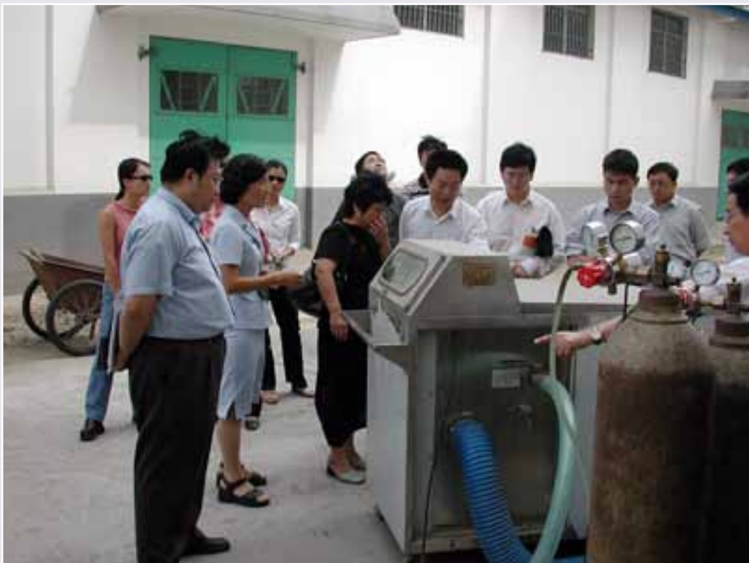
Demonstration of a phosphine fumigant generator to participants at a re-circulation workshop in Xinlong, China
