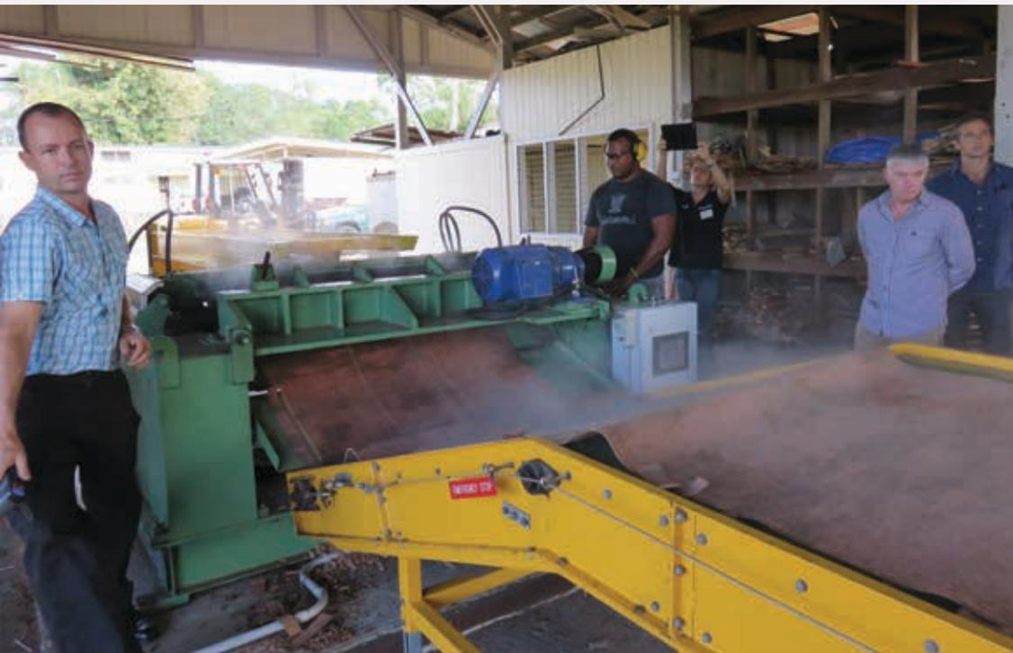
Producing coconut veneer on a spindle-less lathe. Photo: Tony Bartlett.
