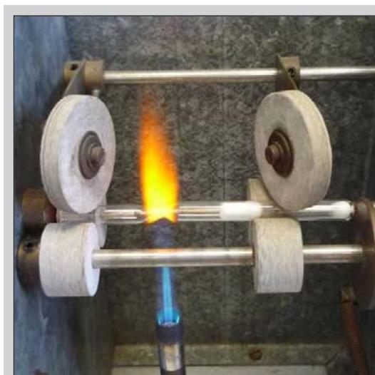
**Figure 4.3** Ampoule constrictor with butane-or propane-fueled flame and angled rollers to assist with stretching of tube for constriction
