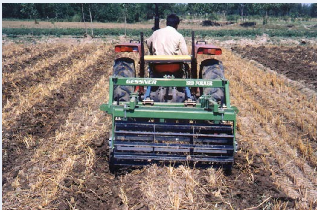
Wide raised bed renovation (Photo: G. Hamilton)
