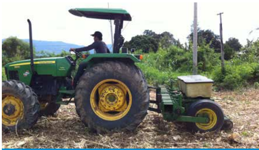
Figure 7. Step 3: no-till planting into 5 t/ha maize residue using a three-row John Deere Maxemerge planter. Photo: R. Martin
