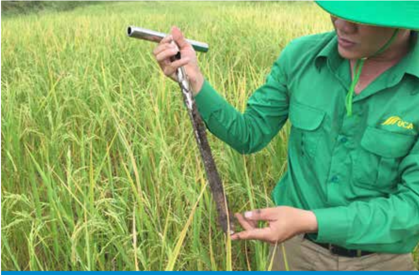
Figure 2. Checking for hard pans on rice soils. Photo: R. Martin
