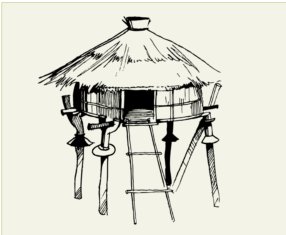
Figure 2. Houses built on poles to raise them well above the ground protect the chickens from predators such as rats, snakes and other wild animals, and dogs. They can also have inverted metal cones around the legs to prevent snakes and rats climbing them.
