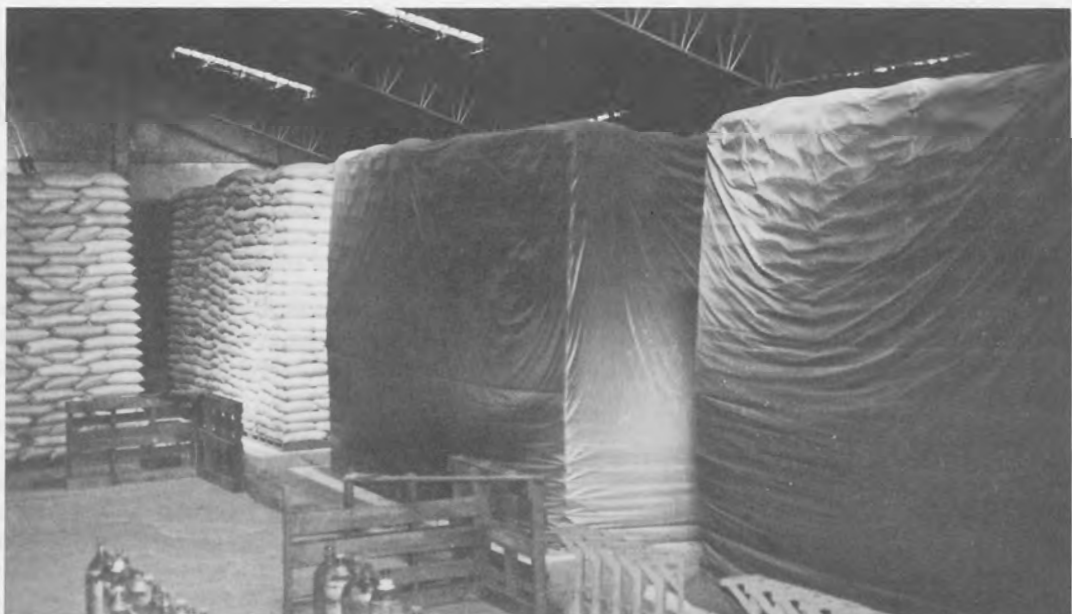
Project 8307 field studies in Southeast Asia began in June 1985. The first trials in the Philippines are on bagged stacks of maize in an NFA warehouse at Cebu City. They are shown here. In the background are the unsealed control stacks.
