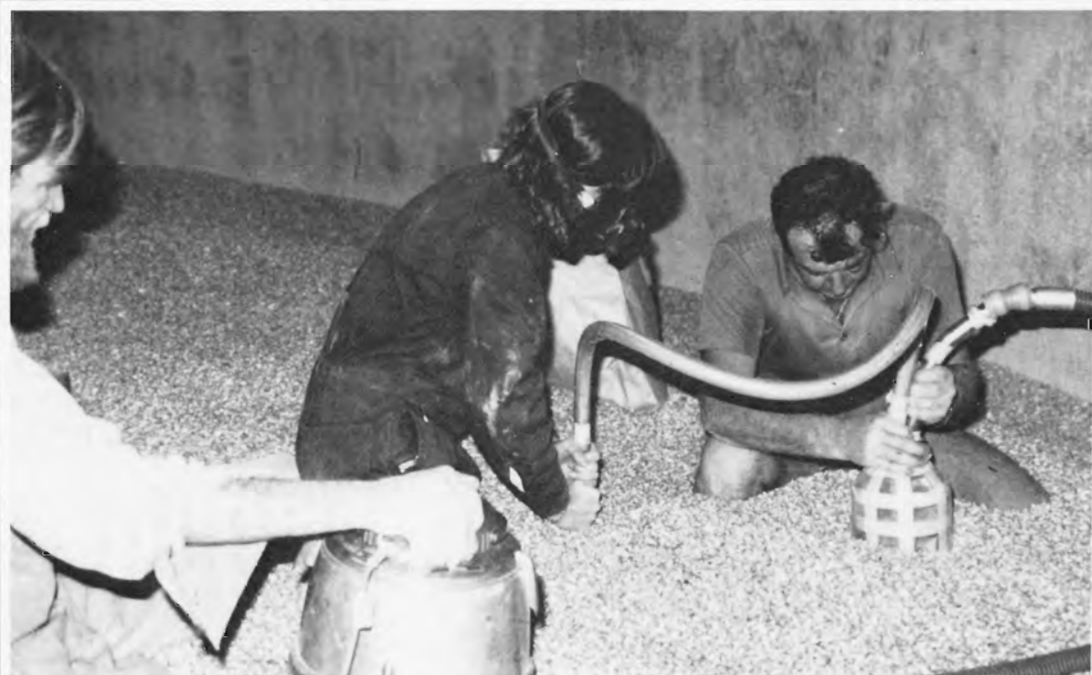
Use of an adapted vacuum cleaner to sample maize treated with protectants at Atherton in the north of Queensland.
