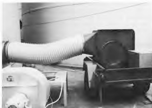
Fig. 15. Mobile unit for natural aeration of grain.
