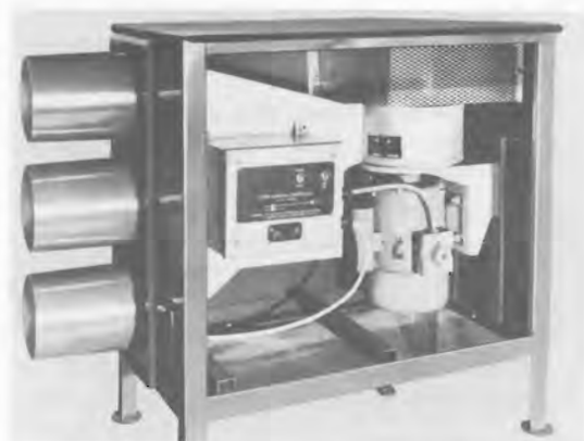
Fig. 4. CSIRO unit for farm aeration of grain.
