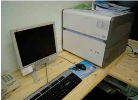
**Figure 2.1** *LightCycler used for real-time PCR is interfaced with computer software to record amplification of DNA over time*
