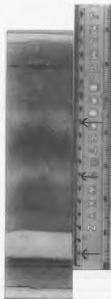
Figure 1. Chromatogram of the crude extract of unripe mangoes, showing the pronounced inhibition zone at R_f 0.10–0.23 (nonresorcinol) and the less pronounced zones at 0.40–0.46 (resorcinols) and 0.66–0.70 (unknown).
