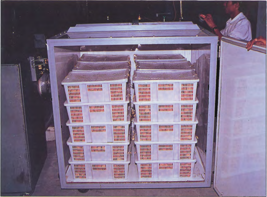
Figure 3. Sulfur dioxide application using a gas fumigation cabinet. This technique is used in Thailand, for both lychee and longan. Gaseous \text{SO}_2 is trickle fed into the sealed chamber to achieve a set internal concentration. Once treatment is complete, \text{SO}_2 is rapidly removed using a large scrubbing chamber, whereby the gas is passed through a fine water mist.
