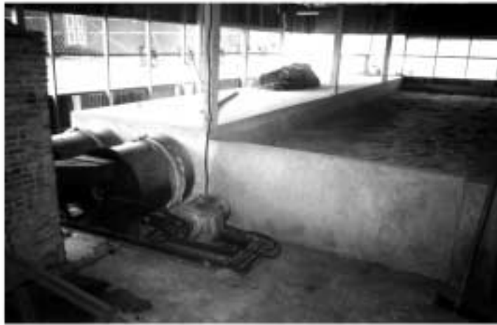
Figure 1. SHG-8 dryer (8 t per 8 hour batch), with side air chamber.
