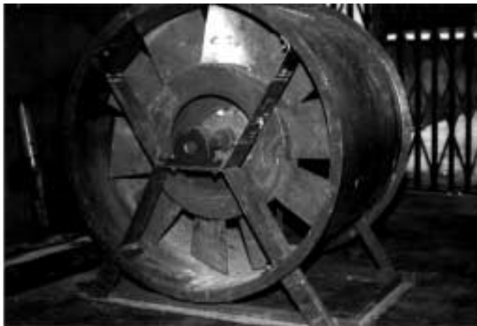
Figure 2. Fan for SHG-4 dryer, with an airflow of 4 m 3 /s at 300 pascal.
