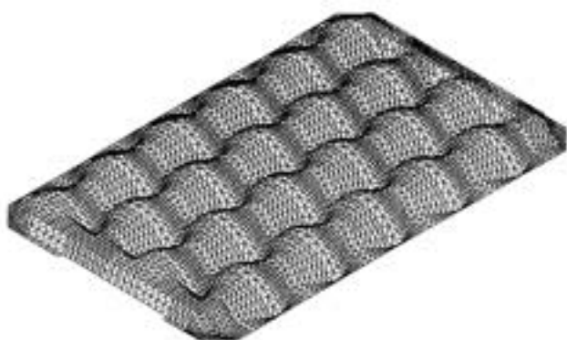
Figure 2. Three-dimensional model of a 'Count 88' tray using two-dimensional elements, without apples.
