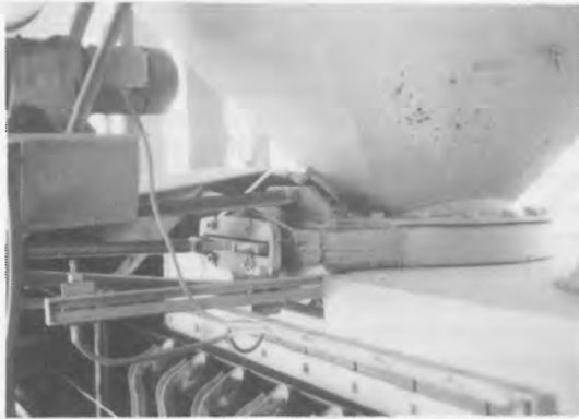
Fig. 15. (a) Gas sealing of discharge valves. (b) Downward clamping of sealing ring around valve plate. (c) Sealing plate in chute below valve. (d) Knife gate valve.
