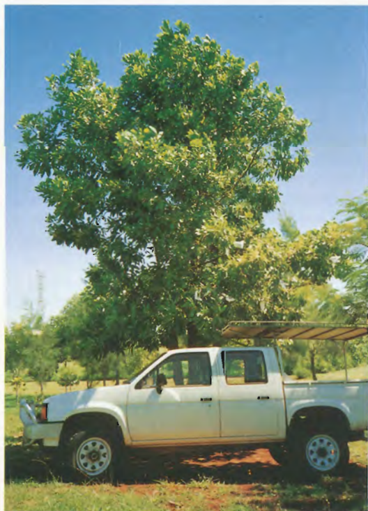
Plate 12 Pollination platform attached to a vehicle.
