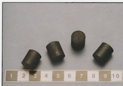
(b) Cobalt pellets (10 g) containing 30% by weight cobaltic oxide in an iron matrix.
