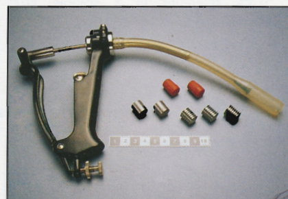
(f) An applicator used to administer cobalt and selenium pellets, steel grub screws and copper oxide capsules to sheep.
