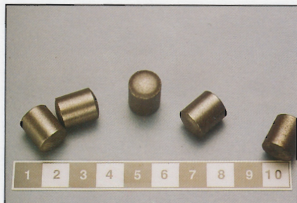
(a) Selenium pellets (10 g) containing 5% by weight elemental selenium in an iron matrix.
