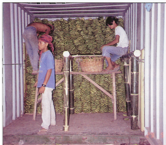
Figure 6. Setting up a trial to evaluate the use of horizontal racks. A horizontal rack running the length of the right-hand half of the van was used.
