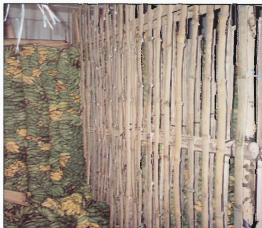
Figure 7. Typical vertical divider now routinely used in bulk shipments of bananas
