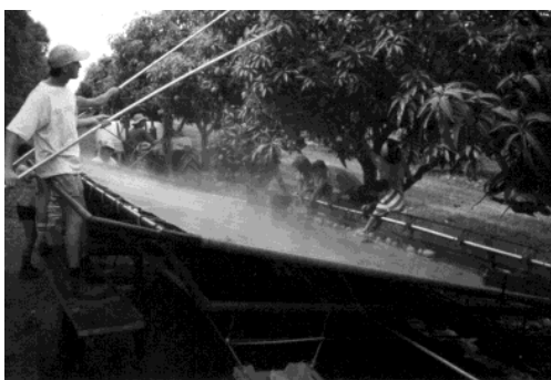
Figure 3. Mango harvest aid reduces sap injury.
