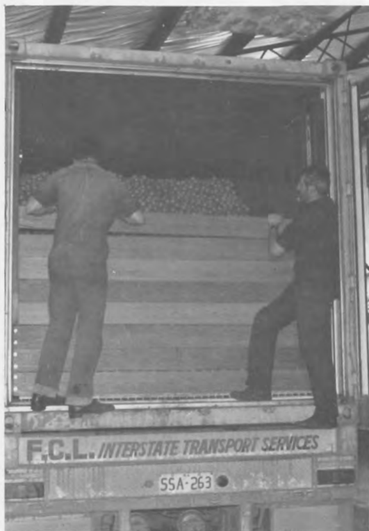
Fig. 2. Bulkhead boards being fitted into channels in doorway.
