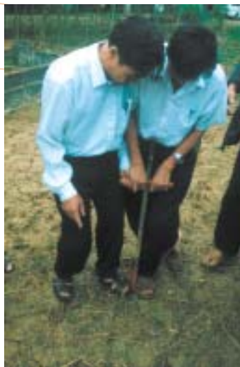
Figure 5.7 Using a soil auger to collect a soil sample in Soc Son district, Vietnam.
