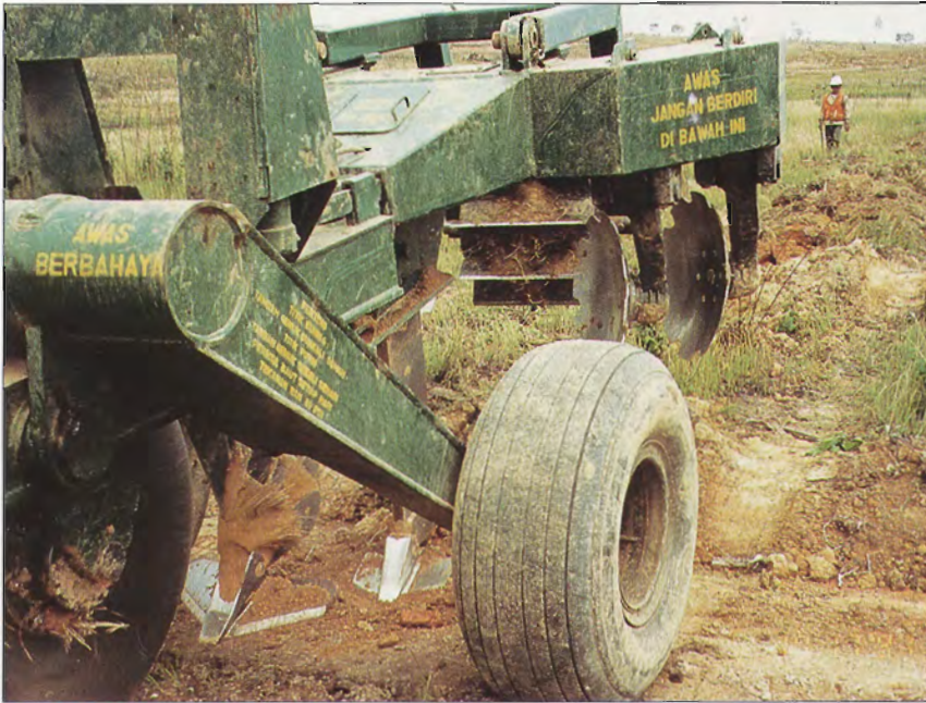
Figure 9. The Savannah 3-in-1 plough. Looking towards the rear of the plough can be seen in sequence the wide winged tip of the blade plough, the tip of the winged deep ripping tyne, the offset discs, and the following tritter wheel.
