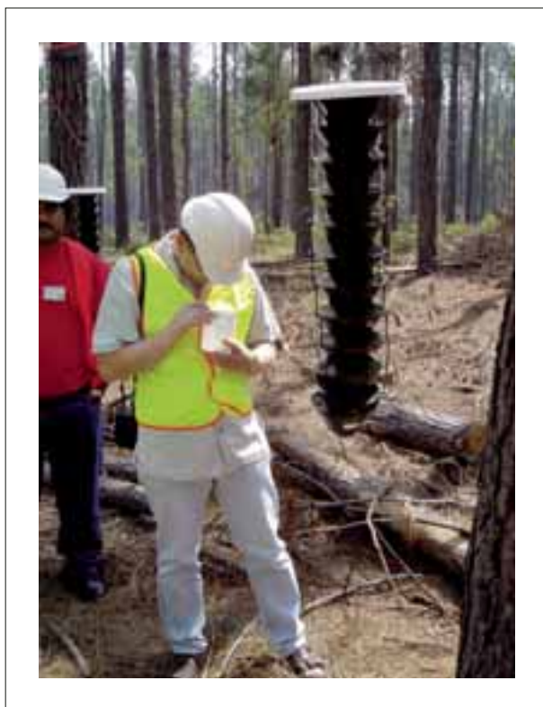
Figure Q5. Static traps using \alpha -pinene as an attractant for Sirex noctilio wood wasp
